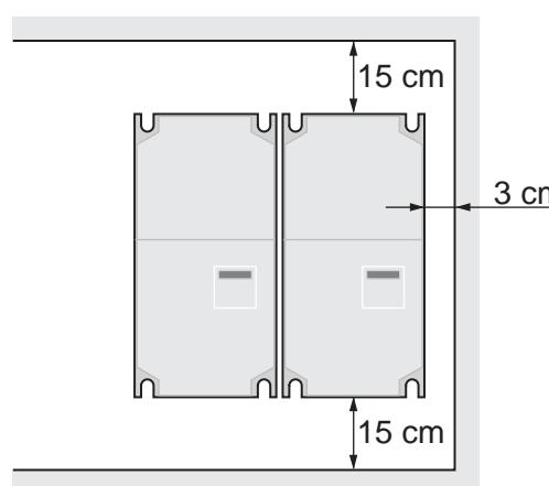
15 cm min. distance at air inlet and air outlet to the next subassembly
