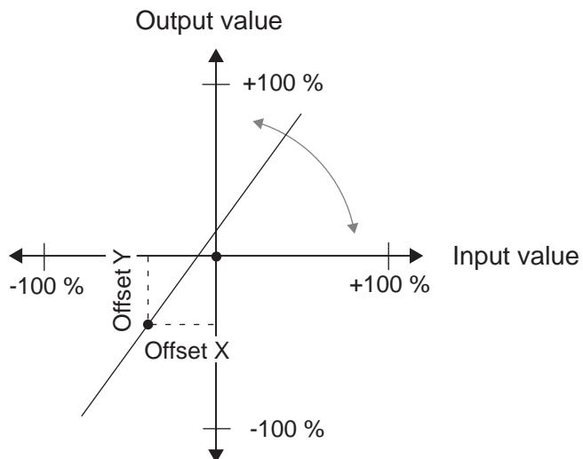
The zeropoint of the characteristic can be defined with offset X (An.16) and offset Y (An.17). In most applications it is sufficient to adjust only one parameter. The rising of the characteristic is determined by the gain.
