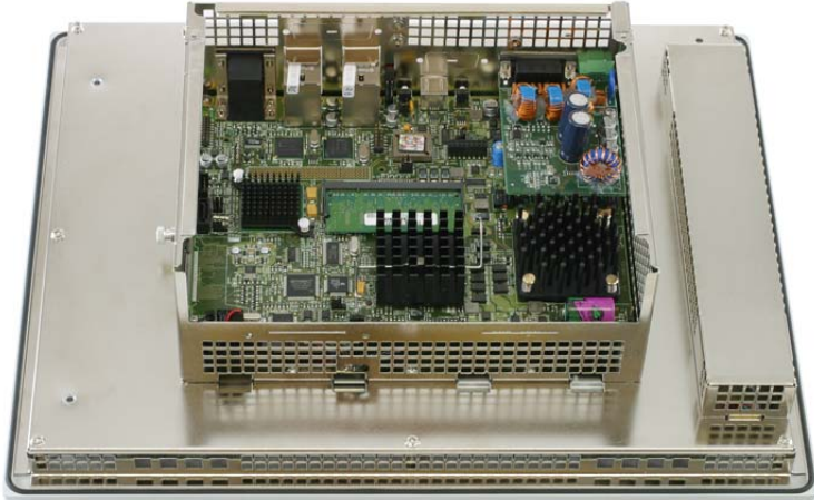
detail of inside of C6 ECON without PCI slot
