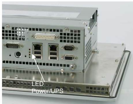
detail of LED of rear panel
