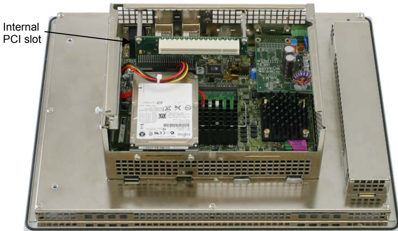
detail of inside of C6 ECON with PCI slot (the PC cell is equipped with a tachometric fan with filter)
