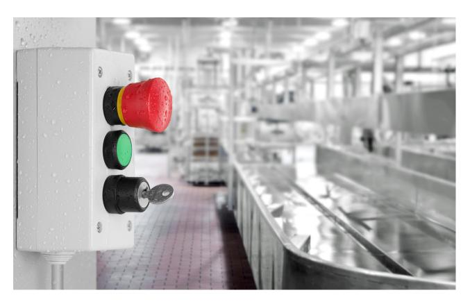
Machines covered by the Machinery Directive (2006/42/EC) must be equipped with at least one emergency stop actuator that can prevent an imminent or occurring hazard.
